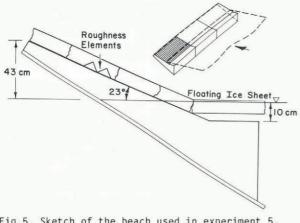
Fig.5. Sketch of the beach used in experiment 5. The left segment of the beach is made rough by triangular wooden pieces.
