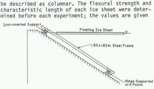
Fig.1. Sketch of steel frame 1.83 m wide.
