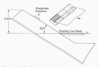
Fig.9. Sketch of the beach used in experiment 12. The left segment of the beach is rough.
