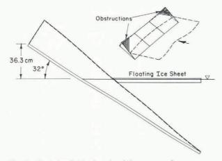
Fig.4. Sketch of the beach with uneven slope and obstructions (experiment 4).
