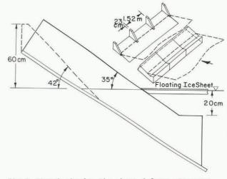
Fig.7. Sketch showing the shore defense structure used in experiment 9 and the beach used in experiment 10.
