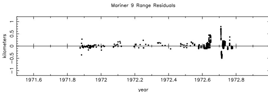
**Figure 4.** Ranging residuals from the Mariner 9 Spacecraft, 1971–72. Much of the scatter is less than 50 m until the times approaching conjunction when the signal passed through the noisy solar corona.
