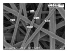
Figure 1. Scanning electron photomicrograph of electropsun nylon nanofibers developed by eSpin Technologies.
