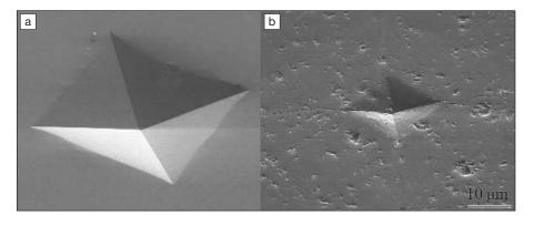
Figure 1. (a) Indentation made in stainless steel by a Vickers indenter; and (b) indentation made with the same indenter and load into  $B_4C$ . The comparatively small indentation mark in  $B_4C$  is an indication of its hardness.
