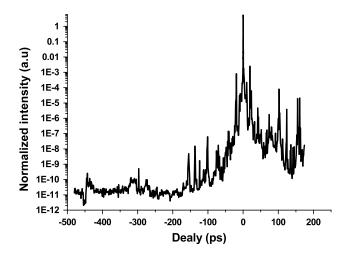
**Figure 6.** Contrast curves of the high-contrast Ti:sapphire CPA laser with a pulse cleaner based on XPW generation<sup>[15]</sup>.
