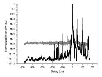
**Figure 4.** Contrast curves of the high-contrast TW-level Ti:sapphire CPA laser (black curve) and the original TW-level Ti:sapphire CPA laser (grey curve). The pre-pulses are identified to be the artefacts generated by multiple reflections at the optical components in the cross-correlator and amplifiers.
