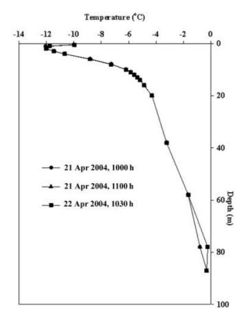
Fig. 1. Borehole temperature profiles measured at 5800 m a.s.l. on the Geladandong icefield, 21 and 22 April 2004.
