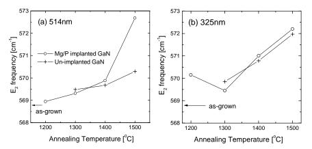
**Figure 2.**  $E_2$  phonon frequency of ion-implanted and of un-implanted GaN films as function of the annealing temperature determined (a) under 514nm- and (b) under 325nm-excitation. The  $E_2$  phonon frequency is a measure for the stress in the GaN.
