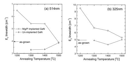
**Figure 1.**  $E_2$  phonon linewidth of ion-implanted and of un-implanted GaN films determined (a) under 514nm- and (b) under 325nm-excitation. The  $E_2$  phonon linewidth is a measure for the crystalline quality of the GaN.
