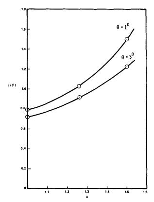
FIGURE 4.—The value of the integral  $I(\theta_0)$  in equation (26) as a function of  $\theta_0$  and  $\alpha$ .
