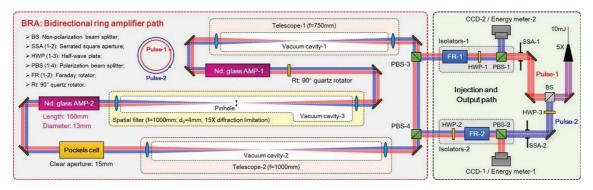
Figure 1. Schematic diagram of the BRA with twin pulses.
