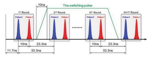
Figure 3. Sequence diagram of the Pockels cell.
