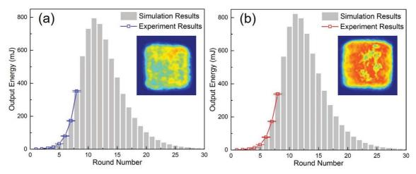
Figure 4. Dependence of the output energy on the number of round trips for single-pulse amplification. (a) Single pulse-1 injected into the RA; (b) single pulse-2 injected into the RA.
