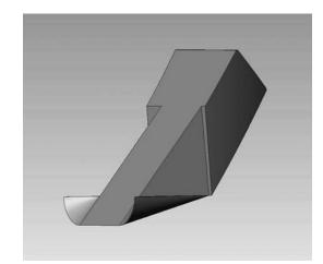
Fig. 5. Sharp-corner cutter.
