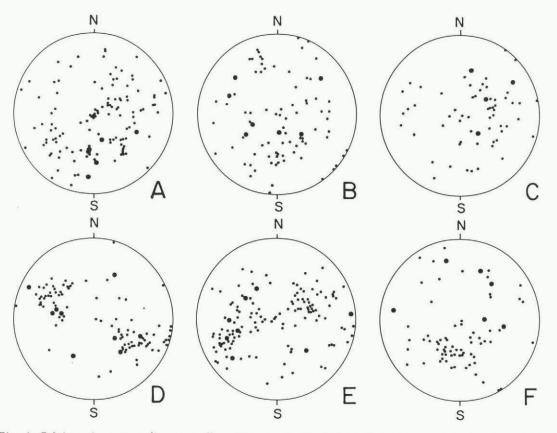
Fig. 6. Fabric point-scatter diagrams illustrating c-axis orientations at (A) 59.52 mbar, (B) 70.71 mbar, (C) 85.28 mbar, (D) 122.65 mbar, (E) 143.18 mbar, and (F) 190.00 mbar. Larger dots represent crystals that are greater than twice the average grain-size.
