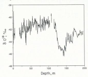
Fig. 7.  $\delta^{18}O_{ICE}$  measurements down-core (50 cm averages).
