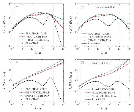
**Figure 4.** Weighted relaxation spectra of non-sheared (a, c) and sheared at 0.01 s<sup>-1</sup> (b, d) PLA-PBAT blend and its nanocomposites with (a, b) 1 wt% and (c, d) 5 wt% clay.
