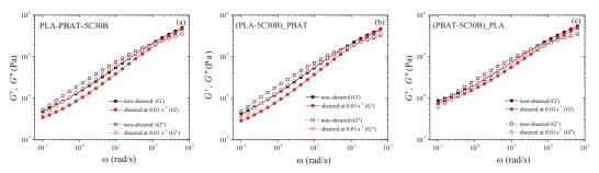
Figure 3. Moduli of non-sheared and sheared nanocomposites with 5 wt% clay prepared via (a) S1, (b) S2, and (c) S3.
