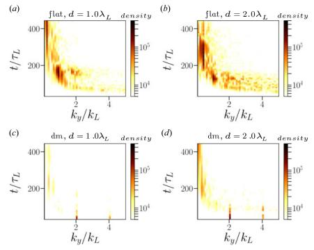
FIGURE 12. Time development  $(t/\tau_L)$  of the FFT of the ion density of a flat target (a,b), and for a density modulated target (c,d) with the normalised wavevector  $k_y/k_L$ . Panels (a,c) and (b,d) are for  $d = 1.0\lambda_L$  and  $d = 2.0\lambda_L$  target widths in respective cases. The modulation parameters are  $a_m = 0.25$ ,  $k_m = 2$ .
