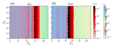
FIGURE 3. Evolution of the ion density and the normalised laser electric field  $a_0$  for (a) a density modulated target ( $k_m = 2$ ,  $a_m = 0.25$ ) and (b) the flat target, for  $a_0 = 150$ . Both targets have  $d = 1.0\lambda_L$  width. The results are shown at  $t/\tau_L = 144$ . The other parameters are the same as in figure 2.
