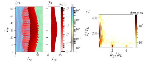
FIGURE 15. Proton density of a target with dm–rpg. The laser pulse has a spatial Gaussian profile with  $a_0 = 150$ . Panel (a) is at  $t/\tau_L = 40$ , while the initial profile at  $t/\tau_L = 0$  is shown in (b). (c) Time development of the FFT of the proton density. Modulation parameters are  $a_m = 0.25$ ,  $k_m = 2$ , and the target widths varies between  $d = 2.0\lambda_L$  and  $d = 1.0\lambda_L$  (see (3.11)). Moving window velocity is  $v_{\text{mov}} = 0.8 c$ .
