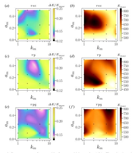
FIGURE 6. Parameter maps for  $a_m$  and  $k_m$  for target thickness  $d = 1.0\lambda_L$ . The colourbars denote  $(a,c,e) \Delta E/E_{\text{max}}$  and  $(b,d,f) E_{\text{max}}$ . Panels (a,b), (c,d) and (e,f) show structured targets viz. (a,b) rec, (c,d) rp, (e,f) rpg, respectively. The other parameters are same as in figure 2.
