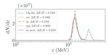
FIGURE 7. Kinetic energy of ions for different targets with modulation parameters  $k_m = 2$ ,  $a_m = 0.25$ , at  $t/\tau_L = 314$  with RR ( $a_0 = 250$ ). The target width is  $d = 1.0\lambda_L$  in each case. Moving window velocities are  $v_{mov} = 0.84c$  for dm target, and  $v_{mov} = 0.8c$  for surface modulated and flat targets.
