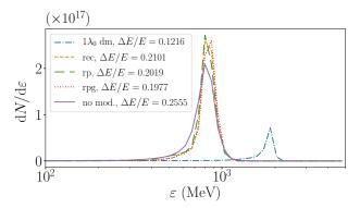
FIGURE 2. Kinetic energy of ions for different targets from figure 1 with modulation parameters,  $k_m = 2$  and  $a_m = 0.25$  at  $t/\tau_L = 440$ . The other parameters are  $a_0 = 150$ ,  $n_e = 250n_c$  and  $d = 1.0\lambda_L$  in each case. The y axis represents the proton numbers, N per unit length. Moving window velocities are  $v_{mov} = 0.8 c$  for dm target, and  $v_{mov} = 0.75 c$  for surface modulated and flat targets.
