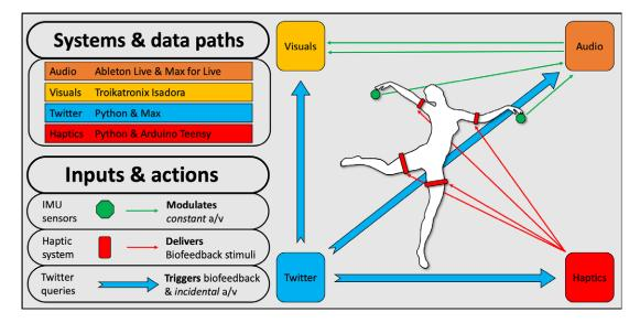
Figure 2. Systems and data paths used for DeviceD.
