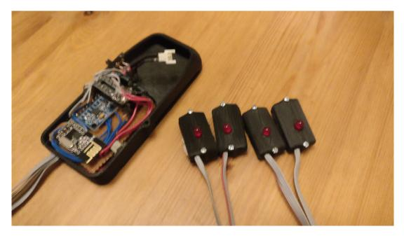
Figure 11. Wearable haptic feedback system, control module (left) and actuators with LEDs (right).
