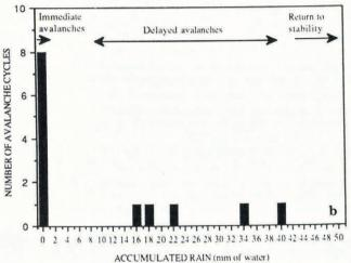
Fig. 1. a. The number and timing of avalanche cycles in relation to the time that rain started. b. The amount of precipitation that had fallen as rain when each of the avalanche cycles occurred. These data are from the eight rain-on-new-snow events that occurred during the winters of 1987-88 and 1988-89.
