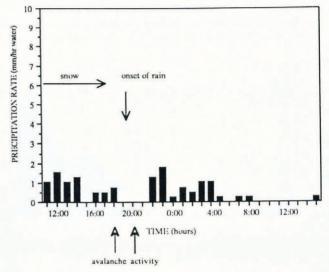
Fig. 5. Hourly measurements at 915 m of air and snow temperatures and precipitation starting at noon on 9 January 1988. Thermistors were buried 24, 34 and 54 cm below the surface. Major avalanche activity (marked by the closed arrow) occurred at the onset of rain but snow temperatures did not warm significantly until about four hours later.
