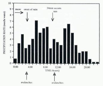
Fig. 6. Hourly measurements at 915 m of air and snow temperatures and precipitation starting at midnight on 14 January 1988. Thermistors were buried 15, 25 and 40 cm below the surface. Closed arrows mark the timing of avalanche activity which occurred at the onset of rain, and again 8 h later. Snow temperatures were well below freezing when avalanches first released, but warming had started when the second avalanche cycle occurred.
