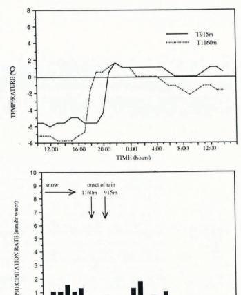
2 16:00 20:(X) 12:00 TIME (hours) avalanche activity Fig. 2. Hourly measurements of air temperature at 915 and
