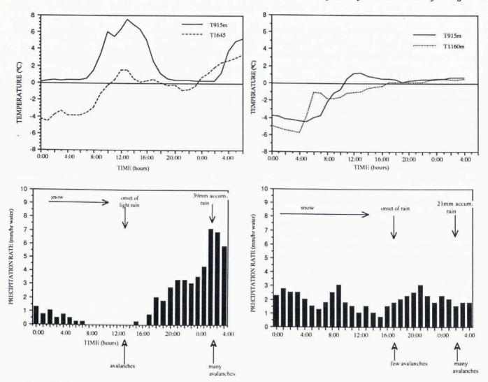
Fig. 3. Hourly measurements of air temperature at 915 and 1645 m and precipitation at 915 m starting at midnight on 4 April 1989. Closed arrows show timing of avalanche activity that occurred first when precipitation changed to rain, and again 13 h later.
