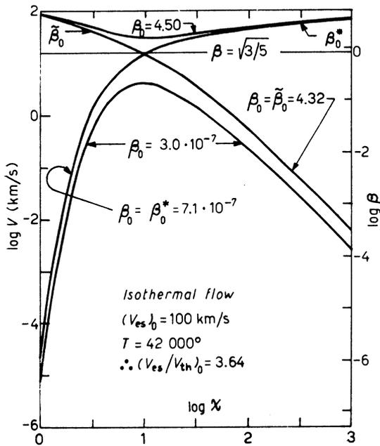
Fig. 6. - The flow velocity  $V$  as a function of  $\chi=r/r_0$ , in four representative isothermal flows. The subsonic flow and the decelerating trans-sonic flow go to zero velocity as  $\chi \rightarrow \infty$ .
