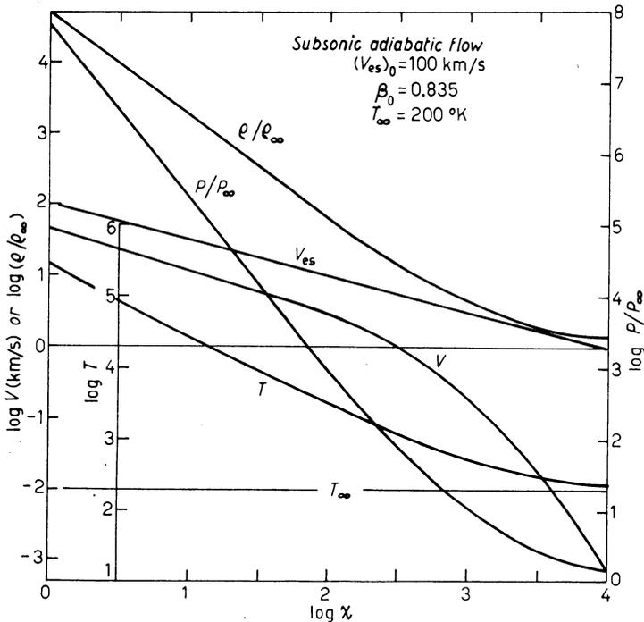
Fig. 9. - A representative subsonic adiabatic flow, with  $\mu = 1.38$ . As  $\chi \rightarrow \infty$ ,  $V \rightarrow 0$ , and the temperature goes to the interstellar value,  $T_I = 200^\circ$ .
