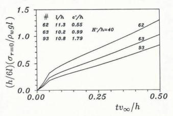
Fig. 5. Maximum radial bending stresses at r' = 0 versus time for test numbers 62, 63 and 93 in Sodhi's experiments.
