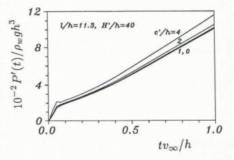
Fig. 4. Influence of the indentor radius on the uplift load.
