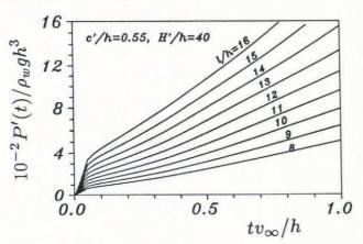
Fig. 3. Influence of the characteristic length on the uplift load.
