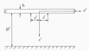
Fig. 1. Problem coordinates and loading configuration. The uplift force exerted by the flat end of the cylinder is approximated by a timedependent ring load.
