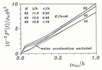
Fig. 2. Uplift load versus time corresponding to the test numbers 62, 63 and 93 in Sodhi's experiments. The dotted lines are applicable if the hydrodynamic reaction is excluded. The foundation is then approximated as a Winkler medium.
