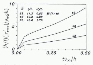
Fig. 6. Average shear stresses at r' = c' versus time for test numbers 62, 63 and 93 in Sodhi's experiments.
