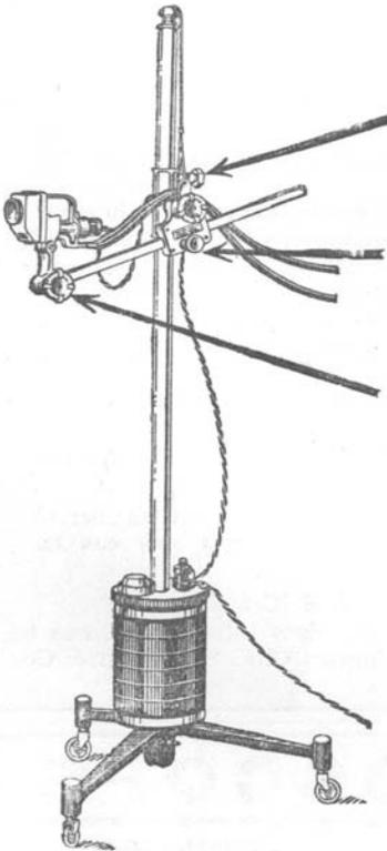
{ Tubular member, for raising or lowering the lamp, attached to an internal counter weight, permitting the lamp to be raised or lowered to any height desired.
