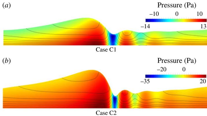
FIGURE 18. (Colour online) Pressure contours and isocontours of the streamwise velocity  $u/u_N \in \{0, 0.1, 0.2, 0.3, 0.5, 0.7, 1, 1.5, 2\}$  in the liquid film of cases C1 and C2, obtained with DNS. In both cases a streamwise section of 0.04 m is shown.
