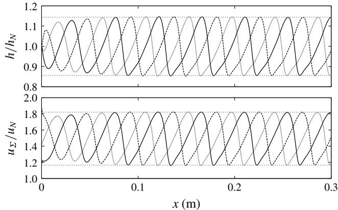
FIGURE 7. Spatial development of the film height  $h/h_N$  and the streamwise velocity at the interface  $u_\Sigma/u_N$  for case A2 ( $Re = 5.2$ ), obtained with DNS. The minimum and maximum values at the measurement position ( $x_m = 0.256$  m) are shown as a reference by the dashed grey lines.
