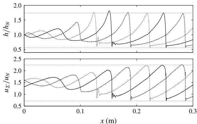
FIGURE 8. Spatial development of the film height  $h/h_N$  and the streamwise velocity at the interface  $u_\Sigma/u_N$  for case C6 ( $Re = 77.0$ ), obtained with DNS. The minimum and maximum values at the measurement position ( $x_m = 0.256$  m) are shown as a reference by the dashed grey lines.
