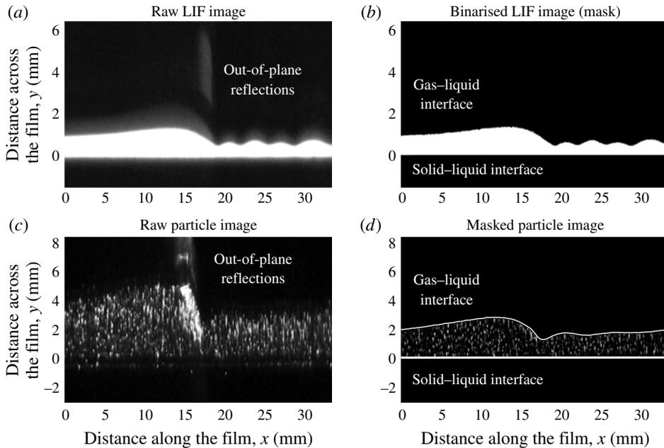
FIGURE 3. (a) PLIF image from a flow with  $Re = 62$ ,  $Ka = 350$  and  $f = 10 \text{ s}^{-1}$ , following corrections for refractive-index and perspective distortions, and (b) binarised PLIF image after removal of out-of-plane reflections. (c) Particle image from a flow with  $Re = 24$ ,  $Ka = 85$  and  $f = 10 \text{ s}^{-1}$  after corrections for refractive-index and perspective distortions, and (d) masked-particle image using its processed PLIF counterpart.
