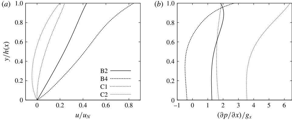
FIGURE 17. DNS profiles of the streamwise velocity  $u/u_N$  (a) and the streamwise pressure gradient (b), normalised with the streamwise component of gravity  $g_x$ , at the trough preceding the solitary wave, position X4, for cases B2 ( $Re = 11.7$ ,  $f = 7 \text{ s}^{-1}$ ), B4 ( $Re = 26.9$ ,  $f = 10 \text{ s}^{-1}$ ), C1 ( $Re = 12.4$ ,  $f = 7 \text{ s}^{-1}$ ) and C2 ( $Re = 28.5$ ,  $f = 10 \text{ s}^{-1}$ ), obtained with DNS.
