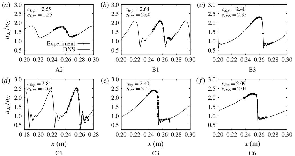
FIGURE 10. Instantaneous streamwise interface velocity  $u_\Sigma$ , normalised with the Nusselt velocity  $u_N$ , for selected cases as a function of downstream distance  $x$ . The wave speeds measured in the experiments,  $c_{Exp}$ , and the DNS,  $c_{DNS}$ , are given as well.
