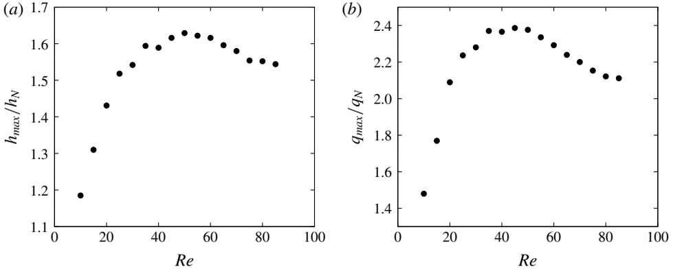
FIGURE 13. Maximum film height  $h_{max}$  (a) and maximum flow rate  $q_{max}$  (b), normalised by the corresponding Nusselt solution, as a function of Reynolds number  $Re$  for case C with  $f = 10 \text{ s}^{-1}$ , obtained with DNS.
