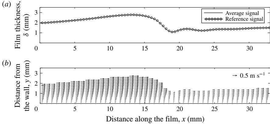
FIGURE 4. (a) Reference and average-wave profiles for a film with  $Re = 26.9$ ,  $Ka = 85$  and a  $10 \text{ s}^{-1}$  forcing frequency. (b) Average PTV-derived velocity field corresponding to the average film-thickness profile in (a).
