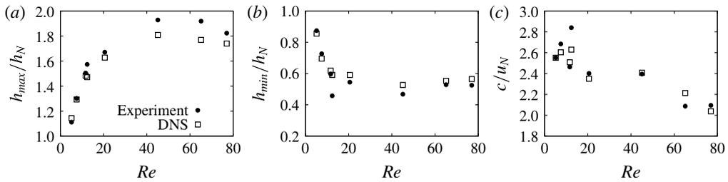
FIGURE 11. Maximum film height  $h_{max}/h_N$  (a), minimum film height  $h_{min}/h_N$  (b) and wave speed  $c/u_N$  (c) as a function of  $Re$  for cases with  $f = 7 \text{ s}^{-1}$ . Results obtained with the LD model are omitted in the interest of clarity.
