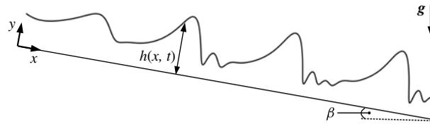
FIGURE 1. Sketch of the profile geometry for a liquid film on a substrate with inclination angle  $\beta$  to the horizontal.  $h(x, t)$  is the local film thickness with respect to a Cartesian coordinate system  $(x, y)$ , with  $x$  the streamwise coordinate and  $y$  the outward-pointing coordinate normal to the substrate.
