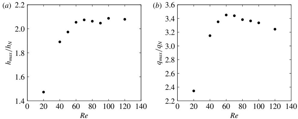
FIGURE 14. Maximum film height  $h_{max}$  (a) and maximum flow rate  $q_{max}$  (b), normalised by the corresponding Nusselt solution, as a function of Reynolds number  $Re$  for a falling water film on a vertical substrate, as previously considered in Denner *et al.* (2016), obtained with DNS.
