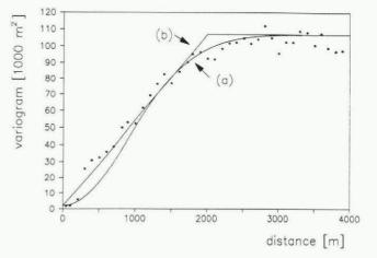
Fig. 6. Variogram of Scharffenbergbotnen subglacial bed topography. \*, experimental variogram; a, Gaussian variogram with parameters nugget effect =  $2000 \text{ m}^2$ , sill =  $105\ 000\ \text{m}^2$ , range =  $2200\ \text{m}$ ; b, linear variogram with sill, with parameters nugget effect =  $2000\ \text{m}^2$ , sill =  $105\ 000\ \text{m}^2$ , range =  $2200\ \text{m}$ . The Gaussian model is preferred because of its better fit, in particular near the origin.
