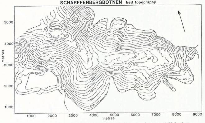
Fig. 3. Subglacial bed topography of Scharffenbergbotnen basin, contoured from a DTM based on universal kriging of radio-echo soundings, using a Gaussian variogram with parameters nugget effect =  $2000 \text{ m}^2$ , sill =  $105\ 000 \text{ m}^2$ , range = 2200 m (see (a) in Fig. 6).
