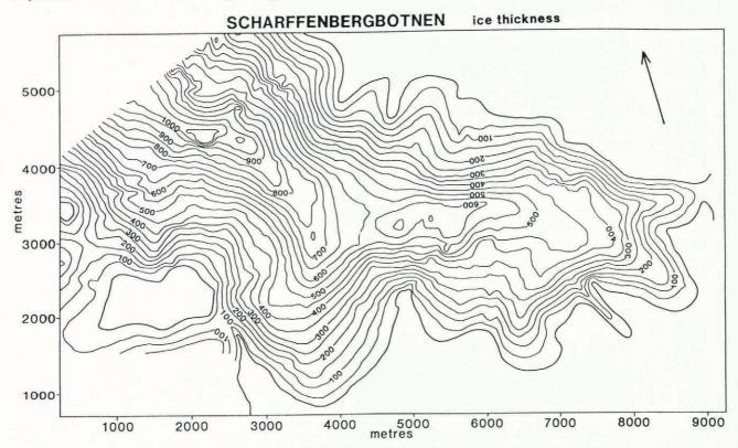
Fig. 2. Ice thickness in Scharffenbergbotnen basin, contoured from a DTM based on universal kriging of radio-echo soundings, using a spherical variogram with parameters nugget effect =  $2000 \text{ m}^2$ , sill =  $78\ 000 \text{ m}^2$ , range = 2500 m (see Fig. 5).
