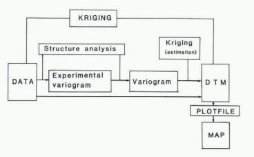
Fig. 4. Diagram of the kriging procedure.
