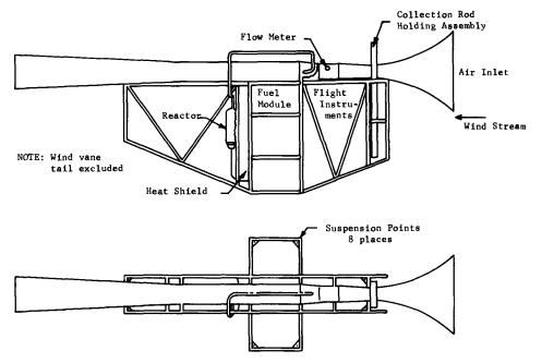
FIGURE 1.—Collector schematic diagram.
