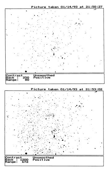
Figure 2. Test images of the Orion area obtained with slightly defocused 8.0 mm lens (f=8.0 mm, 1:1.6) and SBIG ST-6 CCD camera. The field-of-view is roughly 48 x 40  $deg^2$ . (a) Exposure 1 sec. (b) Exposure 9 sec.
