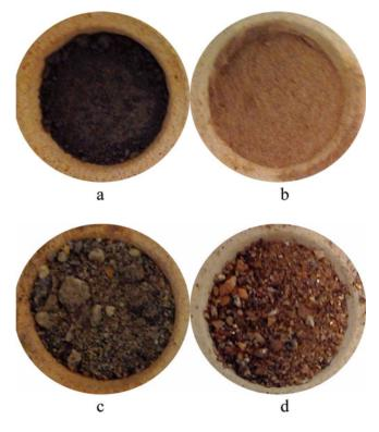
**Fig. 8.** Photographs of the material sampled from (a, b) the Greenland site and (c, d) the Antarctic site in the crucible (a, c) before and (b, d) after the combustion. The diameter of each crucible is 1.25 cm.
