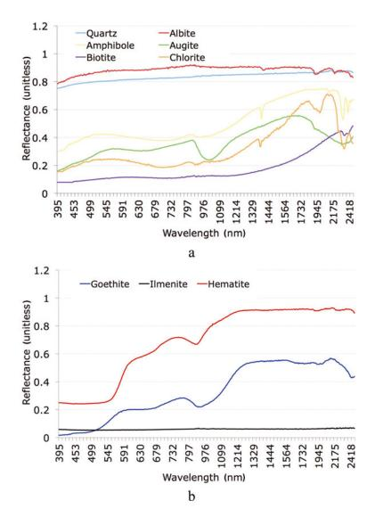
Fig. 7. Examples of reflectance spectra (400–2500 nm) for (a) minerals with a percentage difference between the Greenland and Antarctic samples that is substantial and (b) oxides present in the samples or potentially forming after combustion.
