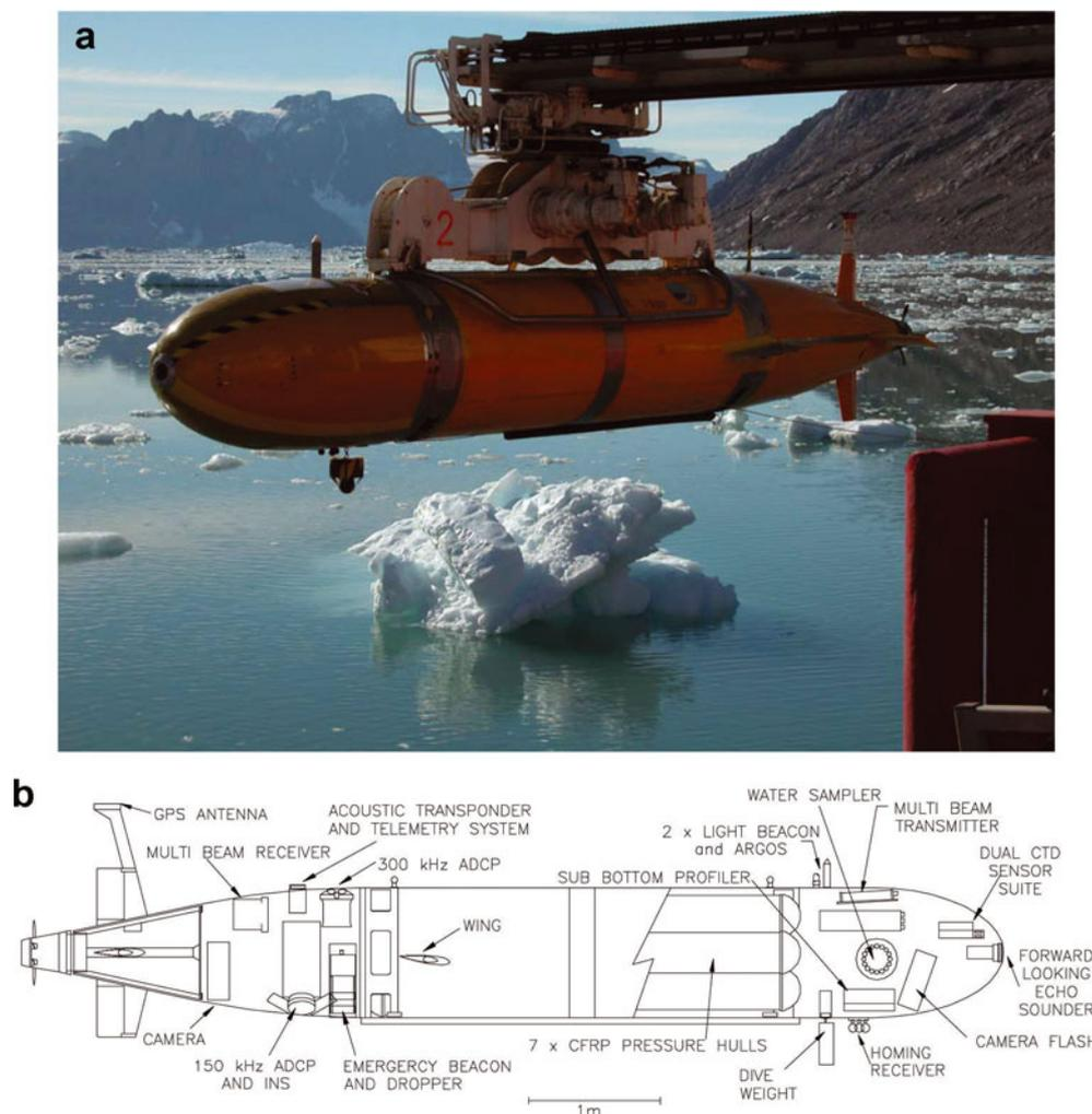
**Fig. 1.** (a) The Autosub AUV being deployed in Courtauld Fjord, East Greenland, from RRS *James Clark Ross*. Autosub is 6.7 m long. Photograph by J.A. Dowdeswell. (b) The major systems of Autosub2 and the science sensors that were installed for the Autosub polar missions of 2003–05. The vehicle displaced 3.6 t and had a range of 400 km at  $1.7 \text{ m s}^{-1}$  with the payload of sensors shown.
