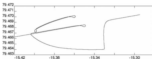
**Fig. 2.** Plan view of collision-avoidance behaviour, triggered by detection of a 30 m deep iceberg keel ahead on mission 365 off northeast Greenland (Wadhams and others, 2006). It took three attempts for Autosub to avoid the hazard and continue eastwards on its programmed course. Axes are in decimal degrees north and west.
