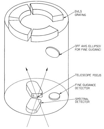
Fig. 1. Schematic layout of the Berkeley spectrograph.
