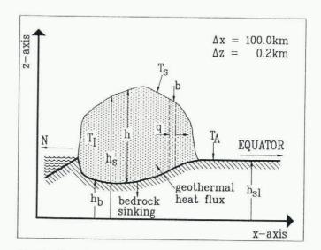
Fig. 1. Coordinate system of the coupled model and definition of model variables used in the text. The resolution of the ice-sheet model is 100 km in the horizontal direction and 200 m in the vertical direction.
