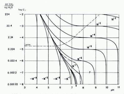
Fig. 3. Total amount of  $CO_2$  in water as a function of pH and the alkalinity as parameter. --- atm: total amount of  $CO_2$  present in the water in equilibrium with the atmosphere (760 torr and 0.033%  $CO_2$ ); --- typical extraction process.
