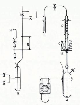
Fig. 1. Apparatus for gas extraction. A: container. B: cooling trap. C: container for ice-water mixture. D: reflux cooler. E: value. F: cooling trap. G: Toepler pump. H: gas sample container. I: grinder.
