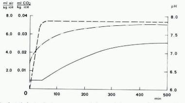
Fig. 2. Results of a typical extraction process. --- total of extracted air; --- total of extracted CO2; --- pH.
