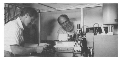
Monte C. Nichols prepares to measure a material sample on the X-ray microanalyzer at Sandia National Laboratories' Livermore, Calif., facilities. Nichols did the conceptual design for the microanalyzer and collaborated on its development with Dale Boehme (left), also with Sandia Livermore, and Richard W. Ryon of Lawrence Livermore National Laboratory.
