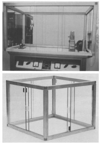
CLEAR-Pb X-ray diffraction enclosure with sliding doors.
