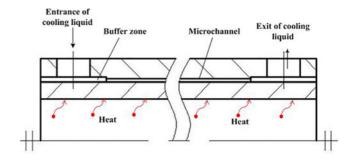
Figure 2. Schematic diagram of microchannel heat sink.
