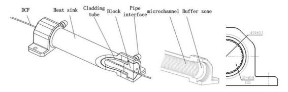
Figure 3. Design of CPS.
