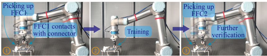
Figure 8. The procedure of the FFC assembly experiment.
