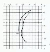
Fig. 4. Temperature of ice in Ha-lung (Halong) glacier: 4900 – bore hole at altitude of 4 900 m, 4500 – bore hole at altitude of 4 500 m.
