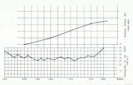
Fig. 6. Above – terminal retreats of 5Y416G4 glacier, 1956–81. Below – thicknesses of ice layers of 5Y564A flattopped glacier of Kakitu.
