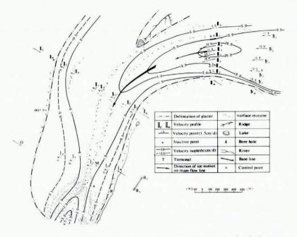
Fig. 1. Isopleth of ice velocity in the lower portion of Ha-lung (Halong) glacier.
