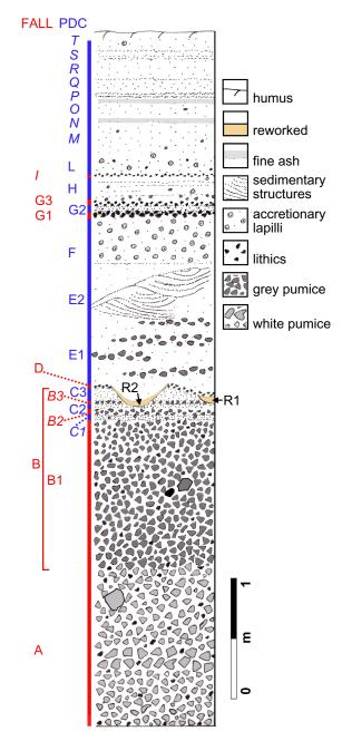
Fig. 2. (Colour online) Composite stratigraphic section showing the maximum thickness of the units of the AD 79 deposit at Pompeii (except for unit E, reaching 3.3 m thickness at one location). On the left, all units are classified as emplaced by fall (in red) or by pyroclastic density currents (PDC) (in blue). Note the presence of two erosive surfaces filled by reworked material under fall layer D (R1) and PDC layer E (R2). Levels described for the first time are formatted in italics.
