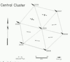
Fig.4. Velocities and strain-rates of the central cluster.
