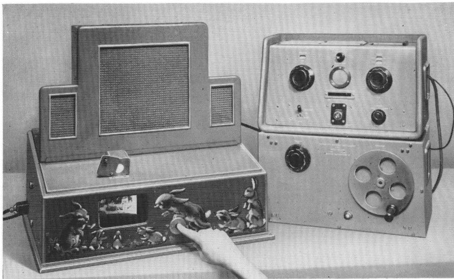
THIS MARCONI AUDIOMETER ASSEMBLY overcomes the familiar difficulties in pure tone audiometry of children. Subject reaction is encouraged by the provision of an interest-feature—a peepshow—which the child quickly learns to operate when the tone is audible, and which is inoperable when no tone is generated. The action of pressing the peepshow button constitutes involuntary acknowledgment of an
