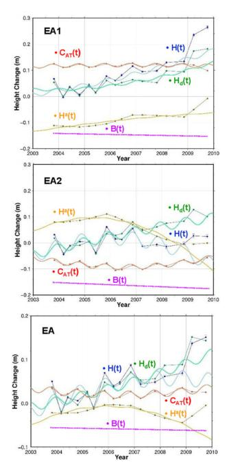
**Fig. 5.** Components of elevation change from ICESat for EA, EA1 and EA2 from  $H_d(t) = H(t) - H^a(t) - C_{AT}(t) - (dB/dt) \times t$  with LQS fit through 2008 data only. Linear trends and the adjusted dB/dt used for B(t) are in Table 3. The dynamic  $H_d(t)$  is more linear than other elevation terms.
