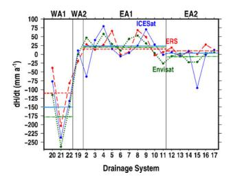
**Fig. 10.** Average dH/dt from ERS1/2 1992–2001 (dashed red), ICESat 2003–2008 (solid blue) and Envisat 2002.7–20010.7 (dotted green) by DS and sub-regions for areas of common coverage. DS20, 21, 22, 19 and 4 to 16 are completely covered.
