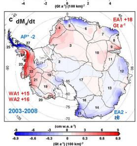
**Fig. 16.** ICESat maps for 2003–2008, (a) dM/dt, (b)  $dM_d/dt$  and (c)  $dM_a/dt$  using dB/dt equal to Ivinsd $B/dt + \delta B_{adj}$ . Rates are linear terms of LQS fits at year 2006.0. \*Rates for AP from average-linear-change analysis.
