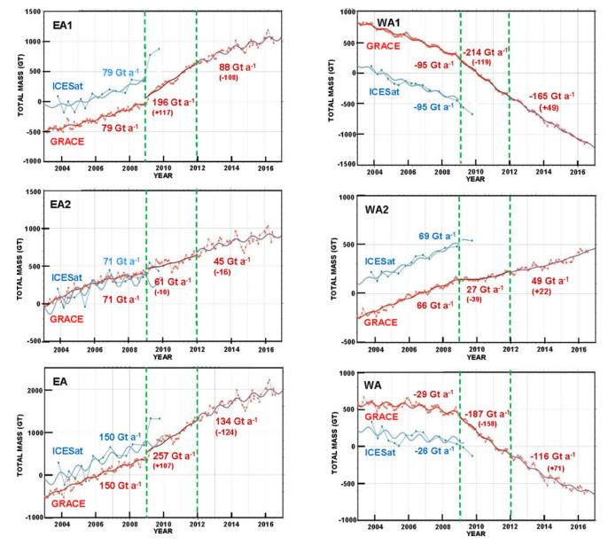
**Fig. 12.** M(t) time series for East Antarctica from ICESat (blue) and GRACE (red) using the equalizing  $dB_{cor}$  and  $GIA_{cor}$  listed in Table 3. The linear trends from LQS fits at the midpoints of 2003–2009, 2009–2012 and 2012–2016.3 also in Table 7a.
