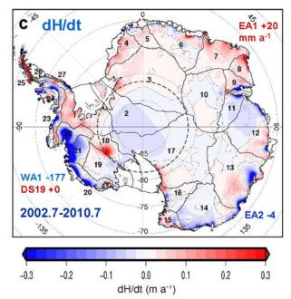
**Fig. 9.** Maps of dH/dt: (a) for 1992–2001 from ERS1/2, (b) for 2003–2008 from ICESat, and (c) for 2002.7–2010.7 from Envisat showing regional dH/dt for areas of common coverage. (Areas south of 81.6° coverage of ERS and Envisat and south of 86° of ICESat are interpolated in images.)
