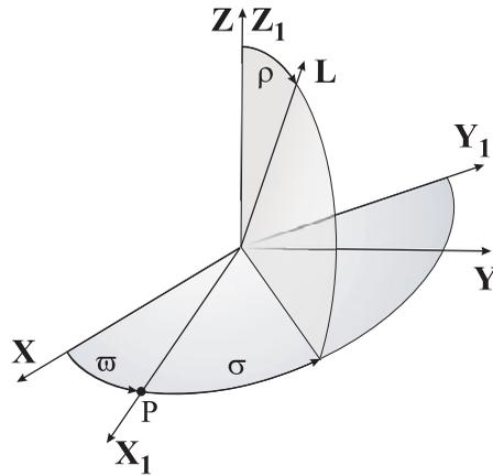
Figure 2. Orientation of kinetic moment vector,  $\vec{L}$ , relative to the pericentre of the orbit, P.
