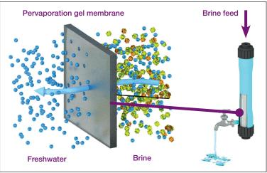
Pervaporation as a promising candidate for brine treatment. The figure shows how composite pervaporation membranes, prepared by coating the surface of PVDF supporting membranes with PVA, are almost completely impermeable to salts. Credit: Vicki Chen and co-workers, University of New South Wales.
