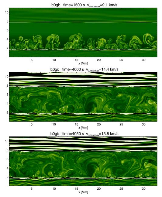
Figure 3. Entropy inhomogeneities for three snapshots of a 2D simulation with a resolution of  $2400 \times 800$  grid points. The horizontal average of the entropy has been subtracted to render small fluctuations visible. A brighter color indicates material with an entropy excess (i.e. lower density than the surroundings). The overturning flow inside the convection zone clearly differs from the oscillatory motions due to gravity waves inside the stable layers.
