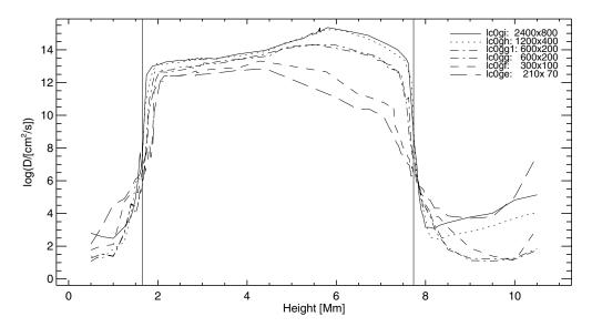
**Figure 4.** Logarithm of the diffusion coefficient versus height for models with different resolutions (indicated in the legend). The two vertical lines mark the boundaries of the entropy plateau at the start of the simulations. Later, they are slightly smeared out. The results from the runs with the two lowest resolutions differ significantly from the runs with next higher resolutions. Nevertheless, the agreement between the two highest-resolution runs is rather good.
