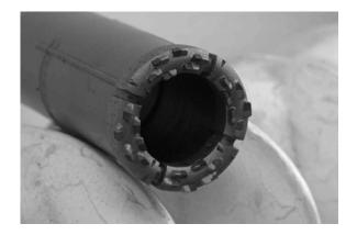
Fig. 5. Temperature-stabilized diamond rock-coring bit.
