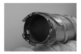
Fig. 2. Koci drill 3 cutter core head.
