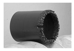
Fig. 4. Crushed carbide rock-coring bit.
