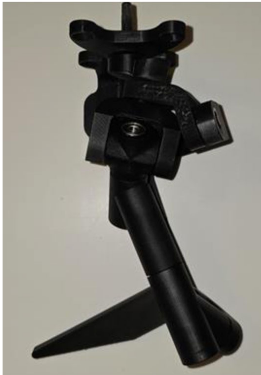
Figure 12. Assembled overconstrained walking mechanism.
