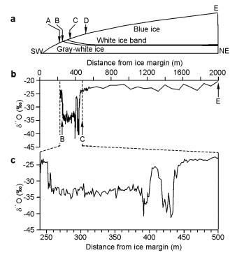
Fig. 2. (a) Schematic southwest–northeast cross-section through the margin of Barnes Ice Cap. A-E are control points on sampling transect. Sampling interval from A to D is 1m, and from D to E is 25m. (b)  $\delta^{18}0$  profile along transect A-E. Segment B–C is enlarged in (c).
