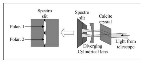
Figure 4. The additional optics to split polarizations and spread the focal spots along the spectrograph slit. A calcite crystal  $(CaC0_3)$  transforms the convergent beam from the telescope into two convergent beams, one with polarization 1, the other with polarization 2. The cylindrical diverging lens spreads the two spots in the direction of the spectrograph slit.
